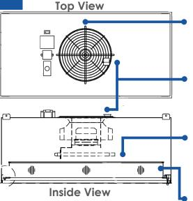
Integrated fan draws unfiltered air into Safe Breathing Zone Unit (SBZU)
