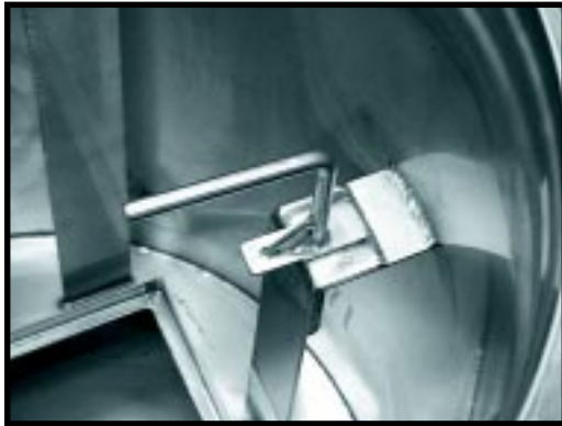
Filter Clamp in locked position without a filter installed.
